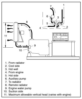
Figure 4-10 Schematic Diagram of Remote Radiator System
